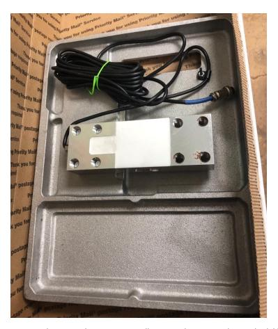
Remove the painted top, using an Allen wrench. Your scale may look like the attached photo. Remove the strain relief next to the carry handle. The wire does not unplug from the load cell. As you can see in photo it does unplug from the indicator end. Notice this photo shows the color code BLUE.
